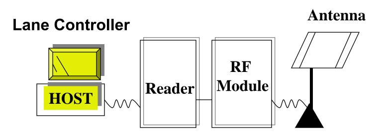
The Host is the Software Database or Lane Controller. Links to the back end computer system. It may be at the site or far a way. The Reader can connect to the Host via Serial Cable, Fiber, Ethernet, Radio or Satellite networks.
