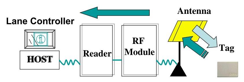
The Antenna captures the Tag ID number, at first as analog RF waves, then it is converted to digital information and send via any mentioned network to the Host computer. Every item may be on site but the Host computer may be remote.
