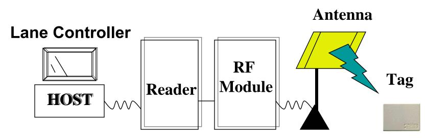
The Antenna is used to broadcast and receive RF signals in the 915-MHz band. Here the Tag is **interrogated** by the Antenna and turns it on. Upon receiving the RF from the Antenna, the Tag then sends its ID back to the Reader through the Antenna.
